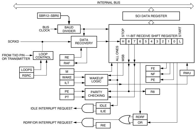
Figure 8-14. SCI Receiver Block Diagram
