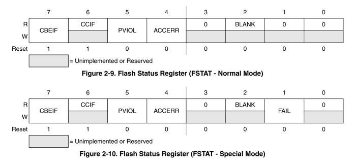
CBEIF, PVIOL, and ACCERR are readable and writable, CCIF and BLANK are readable and not writable, remaining bits read 0and are not writable in normal mode. FAIL is readable and writable in special mode. FAIL must be clear when starting a command write sequence.
