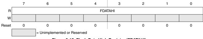
Figure 2-15. Flash Data High Register (FDATAHI)
