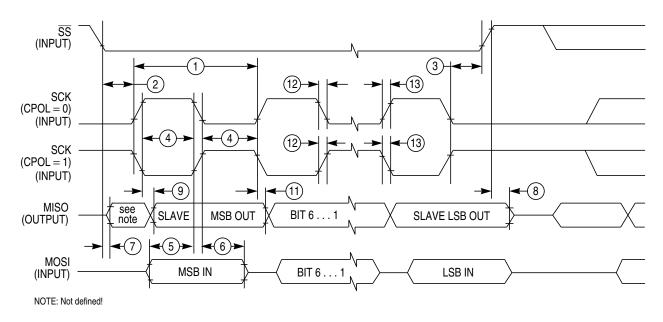
Figure A-14. SPI Slave Timing (CPHA = 1)
