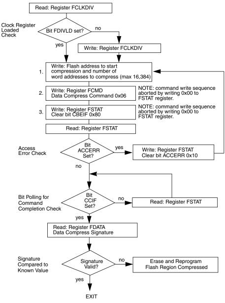
Figure 2-23. Example Data Compress Command Flow
