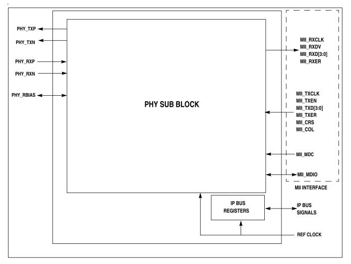
Figure 12-1. Ethernet Physical Transceiver (EPHY) Block Diagram
