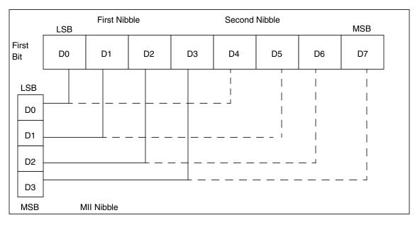
Figure 11-23. MII Nibble/Byte-to-Byte/Nibble Mapping
