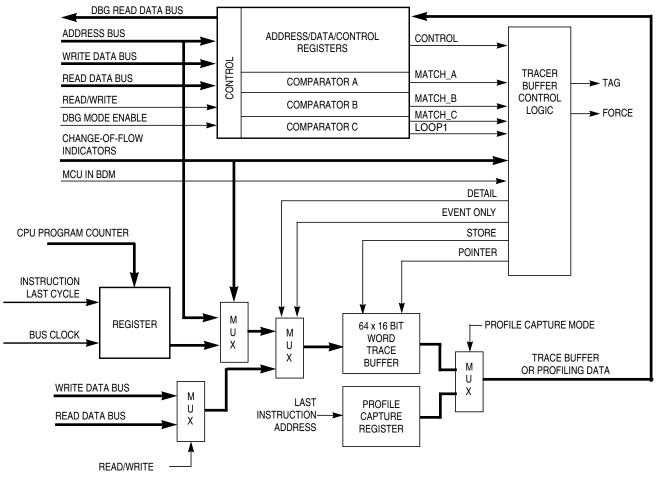
Figure 18-2. DBG Block Diagram in DBG Mode
