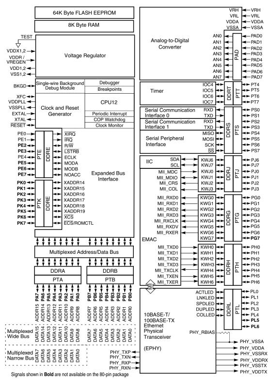
Figure 1-1. MC9S12NE64 Block Diagram
