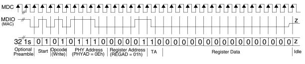
Figure 11-27. Typical MDC/MDIO Write Operation
