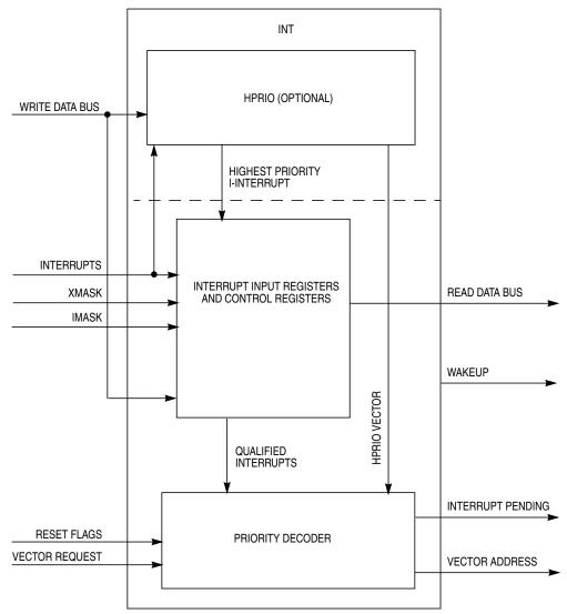
Figure 14-1. INTV1 Block Diagram
