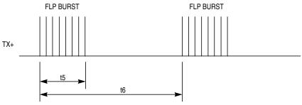
Figure A-8. Fast Link Pulse Timing
