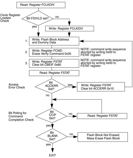
Figure 2-22. Example Erase Verify Command Flow
