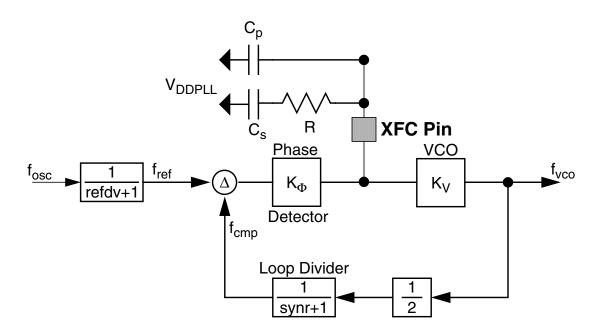
Figure 18-22. Basic PLL Functional Diagram
