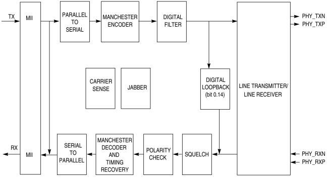
Figure 12-21. 10BASE-T Block Diagram
