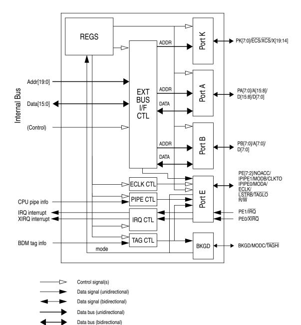
Figure 15-1. MEBI Block Diagram
