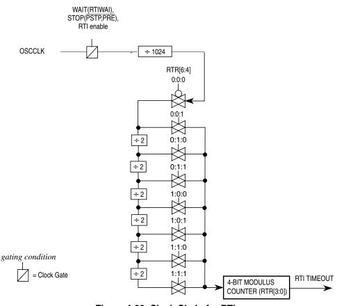
Figure 4-22. Clock Chain for RTI
