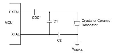
\* Due to the nature of a translated ground Colpitts oscillator a DC voltage bias is applied to the crystal.
