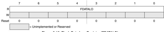
Figure 2-16. Flash Data Low Register (FDATALO)
