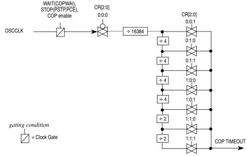
Figure 4-21. Clock Chain for COP
