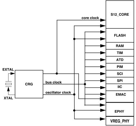
Figure 1-5. Clock Connections
