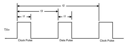
Figure A-9. Auto-Negotiation Pulse Timing
