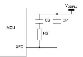
Figure 4-2. PLL Loop Filter Connections
