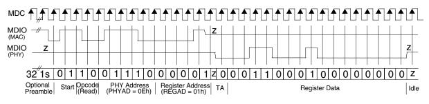
Figure 11-26. Typical MDC/MDIO Read Operation
