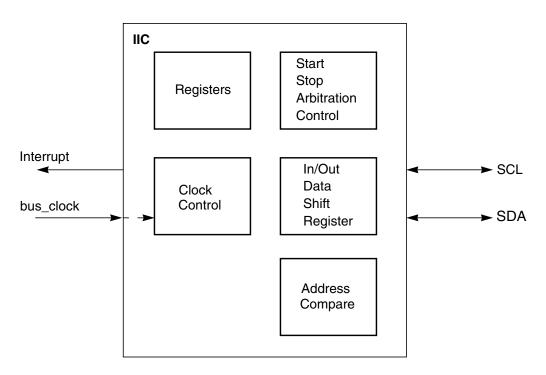
Figure 10-1. IIC Block Diagram
