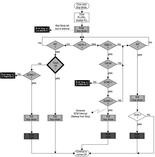
Figure 4-24. Stop Mode Entry/Exit Sequence
