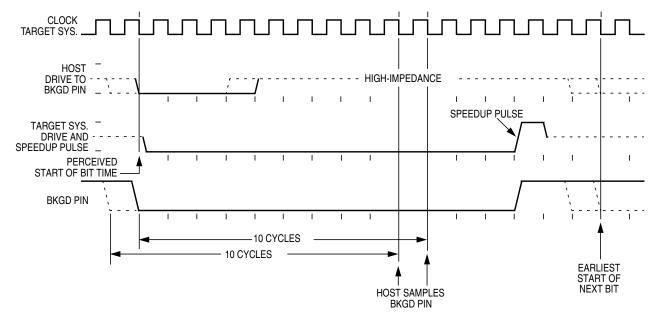
Figure 17-9. BDM Target-to-Host Serial Bit Timing (Logic 0)
