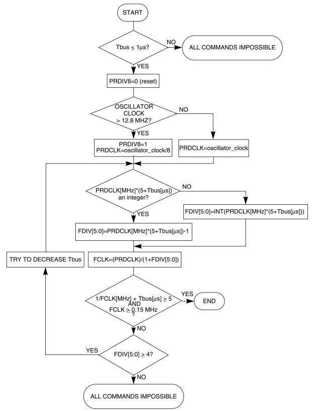
Figure 2-21. Determination Procedure for PRDIV8 and FDIV Bits
