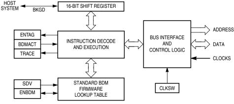
Figure 17-1. BDM Block Diagram
