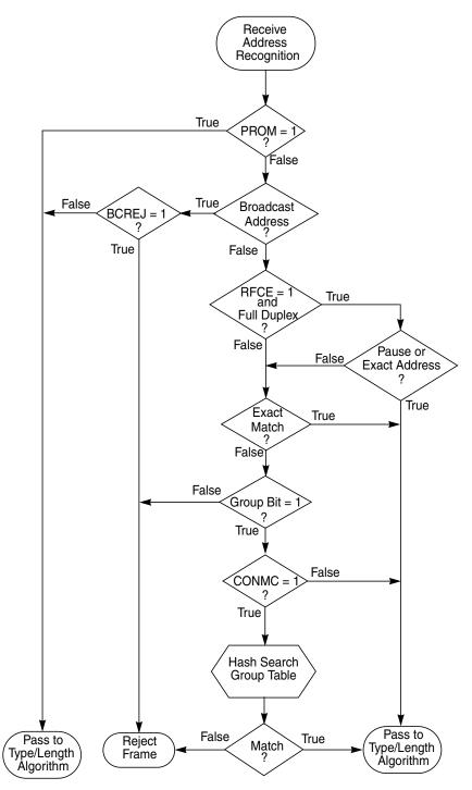
Figure 11-24. Receive Address Recognition Algorithm
