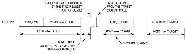
Figure 17-12. ACK Abort Procedure at the Command Level
