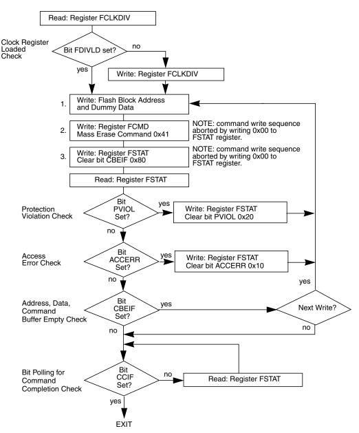
Figure 2-26. Example Mass Erase Command Flow
