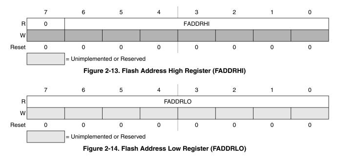
All FADDRHI and FADDRLO bits are readable but are not writable. After an array write as part of a command write sequence, the FADDR registers will contain the mapped MCU address written.
