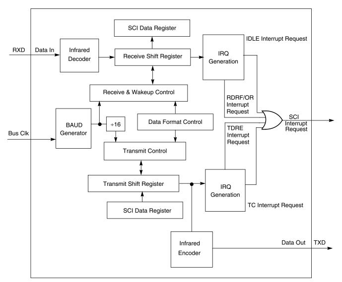
Figure 8-1. SCI Block Diagram
