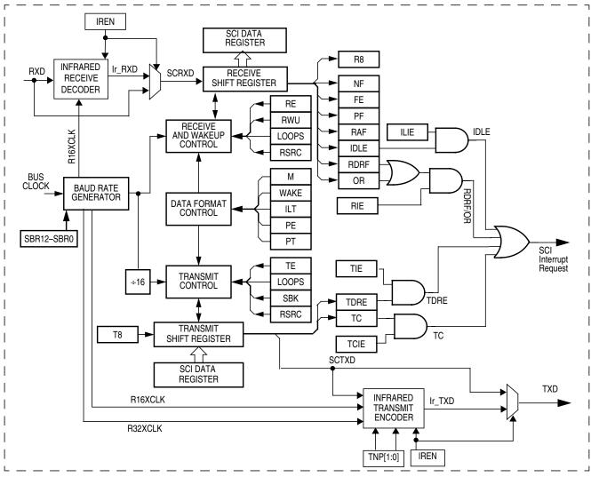
Figure 8-11. Detailed SCI Block Diagram
