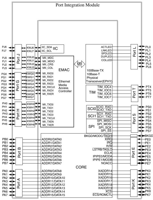
Figure 3-1. PIM\_9NE64 Block Diagram
