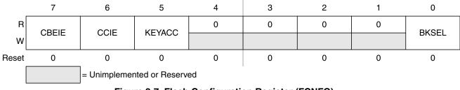
Figure 2-7. Flash Configuration Register (FCNFG)
