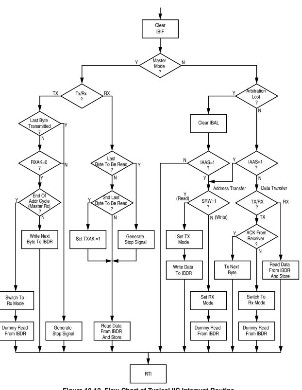
Figure 10-12. Flow-Chart of Typical IIC Interrupt Routine
