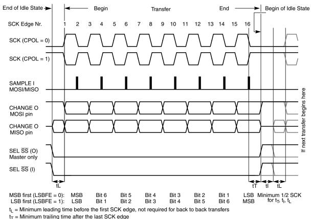
$t_{\rm I}$  = Minimum idling time between transfers (minimum SS high time), not required for back to back transfers
