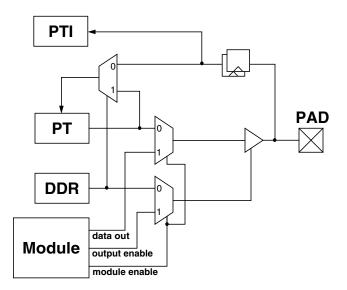
Figure 3-46. Illustration of I/O Pin Functionality
