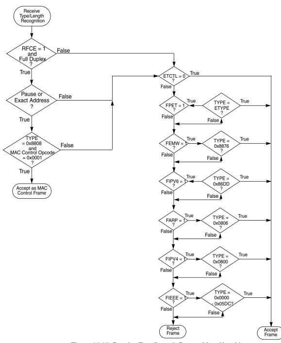
Figure 11-25. Receive Type/Length Recognition Algorithm
