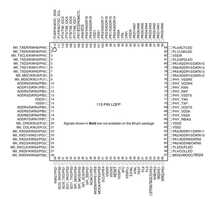
Figure 1-3. Pin Assignments in 112-Pin LQFP for MC9S12NE64
