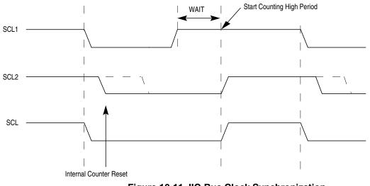
Figure 10-11. IIC-Bus Clock Synchronization
