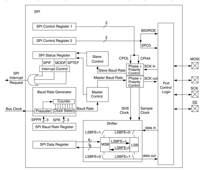
Figure 9-1. SPI Block Diagram
