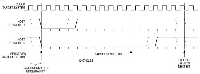
Figure 17-7. BDM Host-to-Target Serial Bit Timing
