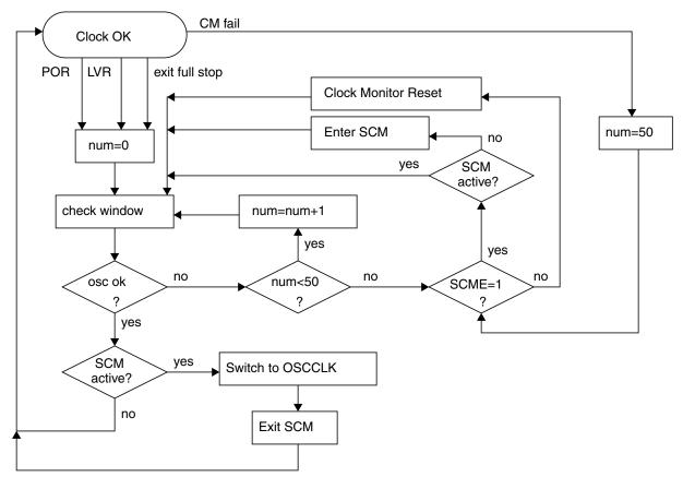
Figure 4-20. Sequence for Clock Quality Check
