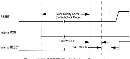
Figure 4-27. RESET Pin Held Low Externally
