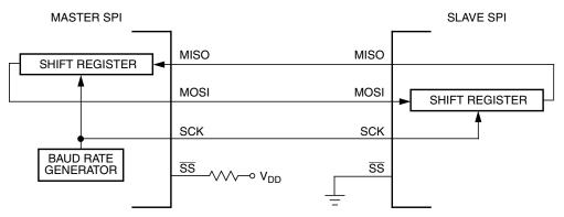
Figure 9-8. Master/Slave Transfer Block Diagram
