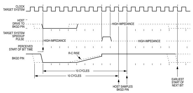
Figure 17-8. BDM Target-to-Host Serial Bit Timing (Logic 1)
