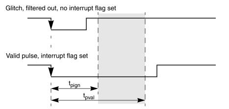
Figure 3-47. Interrupt Glitch Filter on Port G, H, and J (PPS=0)
