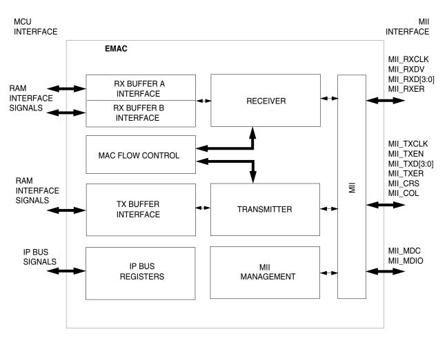
Figure 11-1. EMAC Block Diagram
