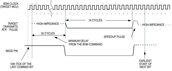
Figure 17-10. Target Acknowledge Pulse (ACK)
