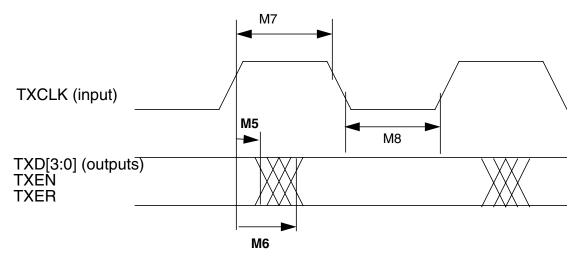
Figure A-2. MII Transmit Signal Timing Diagram
