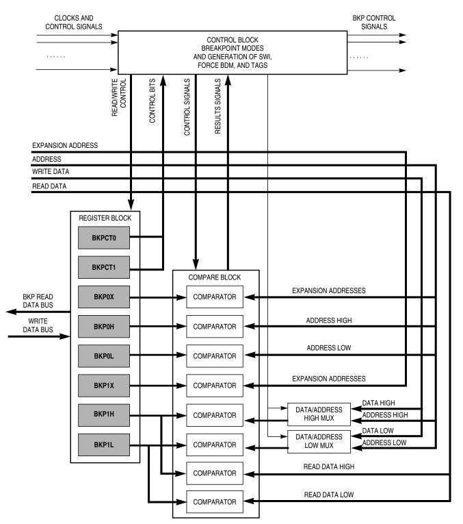
Figure 18-1. DBG Block Diagram in BKP Mode
