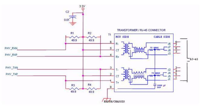
Figure B-2. Ethernet Interface Circuitry
