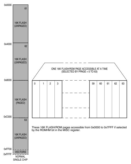
Figure 16-12. Memory Paging Example: 1M Byte On-Chip FLASH/ROM, 64K Allocation
