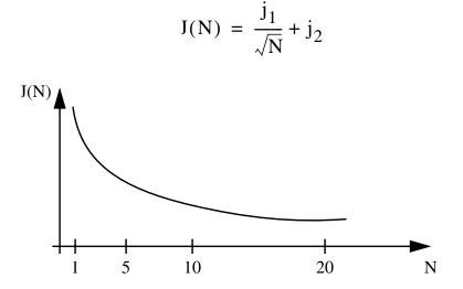
This is very important to notice with respect to timers, serial modules where a prescaler will eliminate the effect of the jitter to a large extent.
