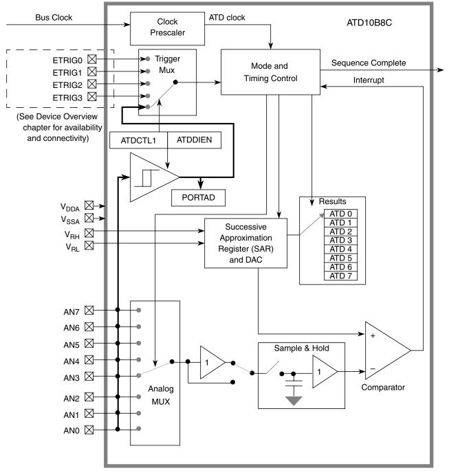
Figure 7-1. ATD Block Diagram
