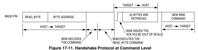
Differently from the normal bit transfer (where the host initiates the transmission), the serial interface ACK handshake pulse is initiated by the target MCU by issuing a falling edge in the BKGD pin. The hardware handshake protocol in Figure 17-10 specifies the timing when the BKGD pin is being driven, so the host should follow this timing constraint in order to avoid the risk of an electrical conflict in the BKGD pin.
