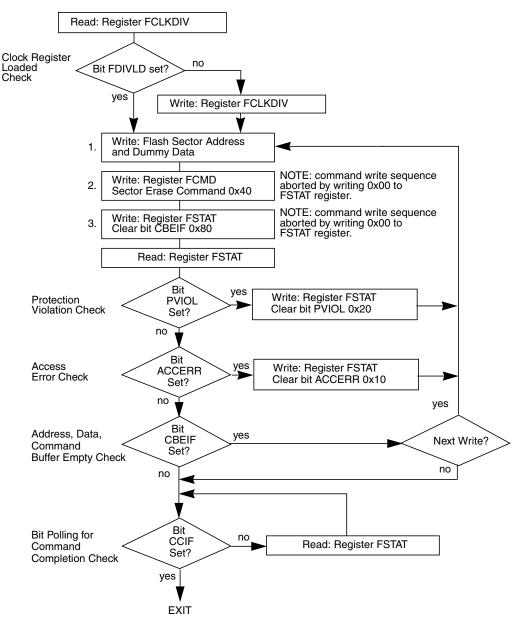
Figure 2-25. Example Sector Erase Command Flow
