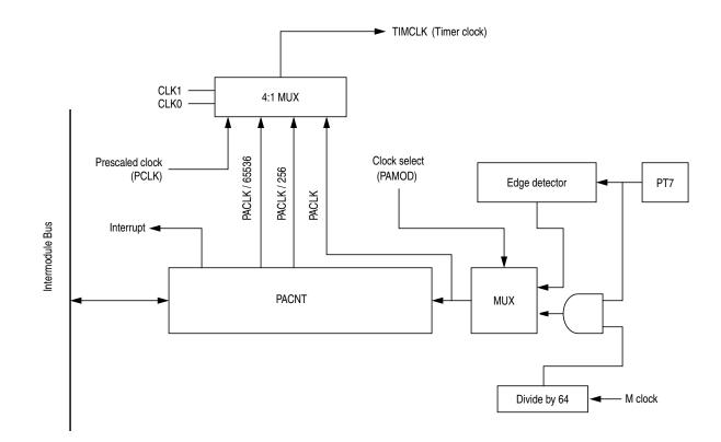
Figure 6-2. 16-Bit Pulse Accumulator Block Diagram
