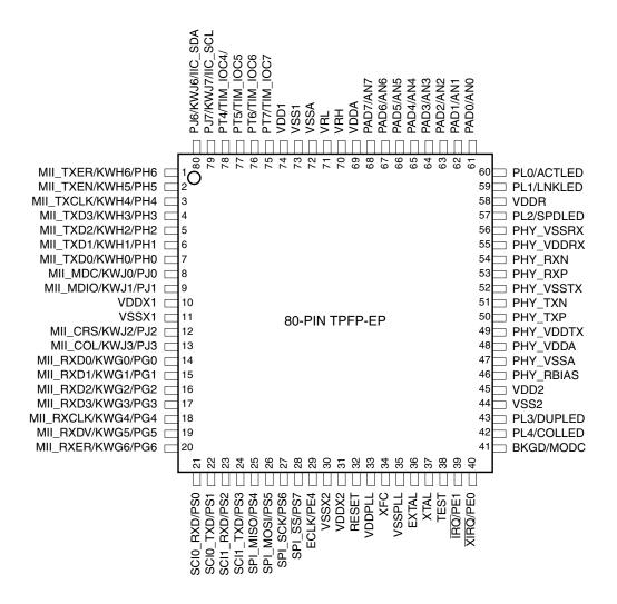
Figure 1-4. Pin Assignments in 80-Pin TQFP-EP for MC9S12NE64
