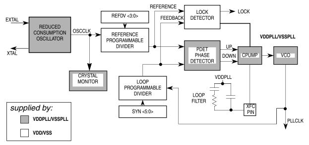
Figure 4-16. PLL Functional Diagram
